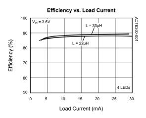
Efficiency vs. Load Current
